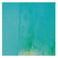
and in cases where the alkalinity is very high, the paint film will actually begin to deteriorate, resulting in premature chipping, flaking or peeling from the substrate. This is most common with oil based and vinyl acrylic paints. Even 100% acrylic paints
