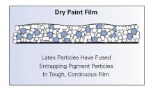
The mechanism of latex paint film formation has some limitations. Because the resin particles are thermoplastic (tending to get softer at higher temperature, and vice-versa), lower temperatures harden the latex particles preventing proper coalescence. In severe cases, this may result in the film actually
